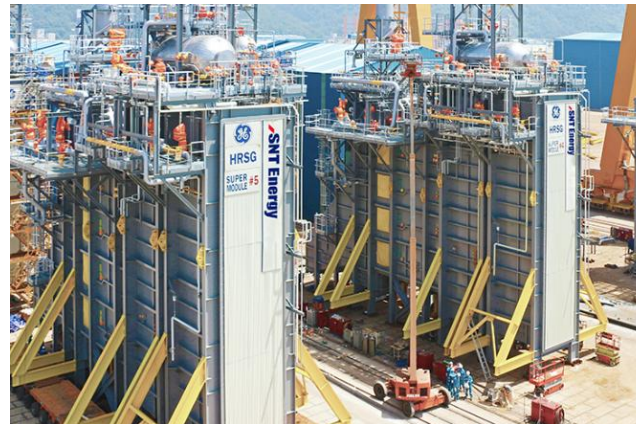
Heat Recovery Steam Generator
