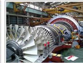
Blade Ring Assembly & Bolt Tightening
